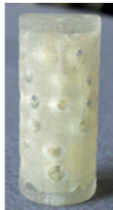
Fig. 2. Specimen before compression test
